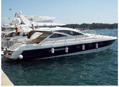
General data: Shipyard and model: GIORGI 50 HARD TOP Length: 15,40 mt Beam: 4,20 mt Displacement: 15000 kg Engines: 2 x Cummins - Linea d'asse - Diesel Power: 2 x 500 Hp (100 h) Fuel Tank: 2x700 lt - Water tank: 440 lt Year of construction: 2009 Load people: 12 people / Berths: 8+2 Cabins: 4 / Bathrooms: 3 CE-category: B - d'altura
