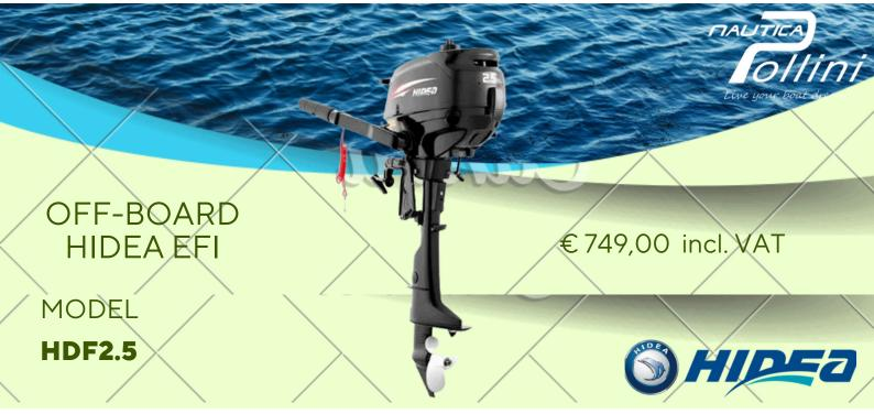
The Hidea HDF2.5 is the smallest engine in the Hidea four stroke range. The HDF2.5 utilizes a single cylinder, water cooled power unit that is extremely compact in its design.
